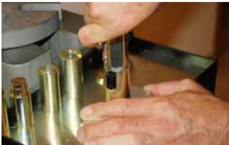
5. Keeping a firm pressure on the tool rotate fully in an anti-clockwise direction followed by 50% clockwise.
