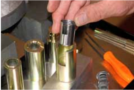
17. Insert the reformed canister into the holding fixture.
