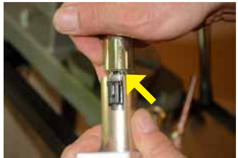
4. Align the main opening tool into the newly opened section to the right of the turret flat.
