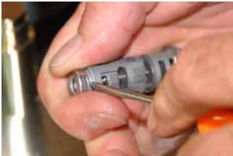
21. Remove turret cap as shown.
