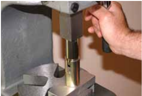
11. Press the tool to reform the canister.
