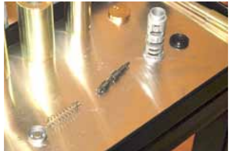
22. Disassemble and clean all parts (Note the direction of rubber seal).
