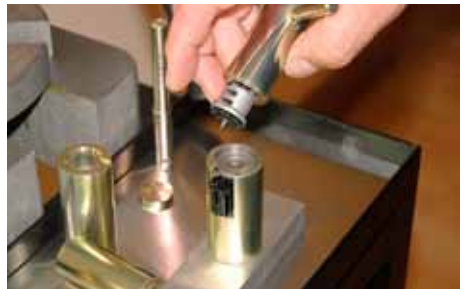
6. Remove the turret section for inspection.
