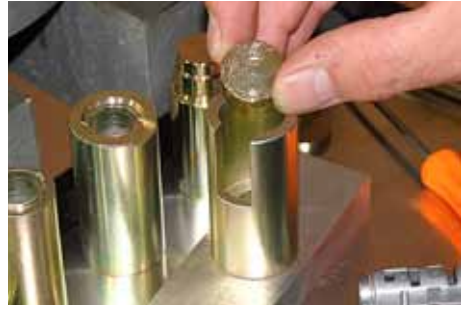
16. Insert spacer A into the holding fixture.
