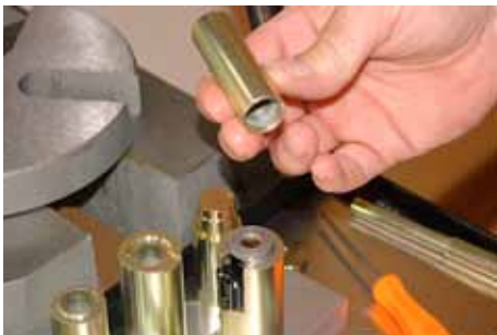
19. Select the tool to push home the internal parts.
