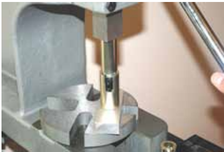
3. Insert into the holding fixture and press down, giving a lead in for the main opening tool.
