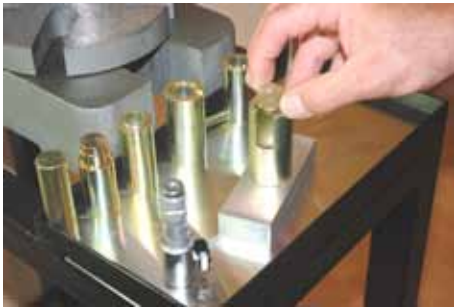
1. Insert spacer A into the holding fixture.
