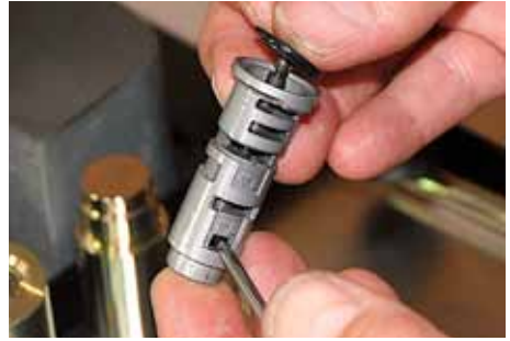
24. Hold valve in place as shown. Refit rubber seal.
