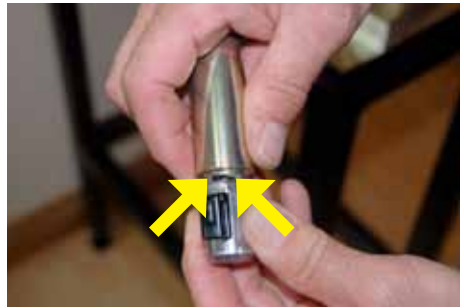
2. Align the initial 2 pin tool either side of turret flat.
