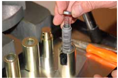
28. Fit the spring and cap.
