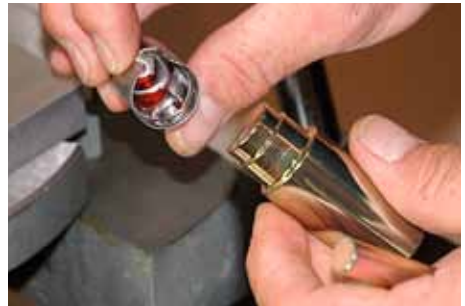
13 & 14. Rotate the canister 180 degrees and repeat this procedure to ensure a perfectly reformed canister.
