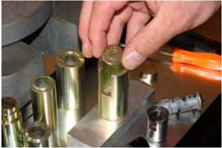
9. Insert spacer B into the holding fixture.
