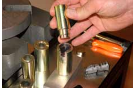
10. Insert the canister and straightening tool into the fixture.
