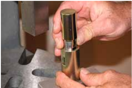
13 & 14. Rotate the canister 180 degrees and repeat this procedure to ensure a perfectly reformed canister.
